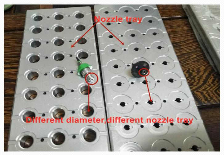
From the picture above, we can see the JUKI nozzle and FUJI nozzle use different fixtures
